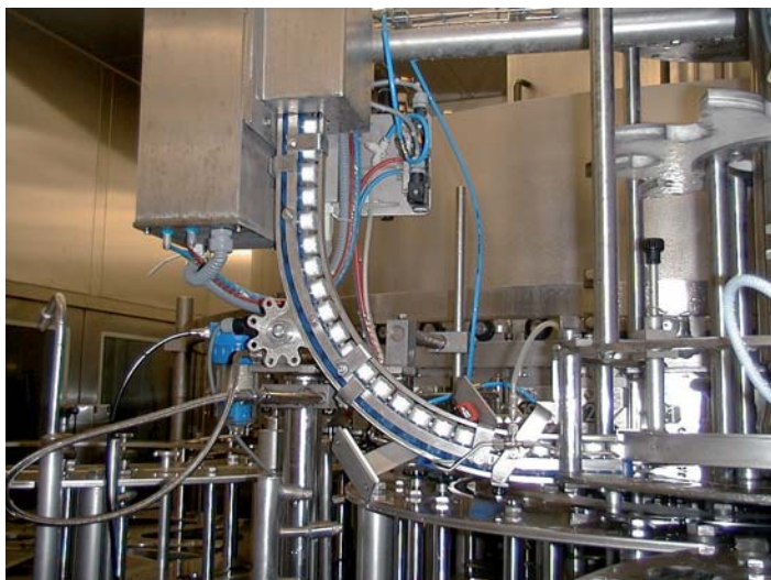
UVATEC used for the disinfection of screw caps in the beverage industry
