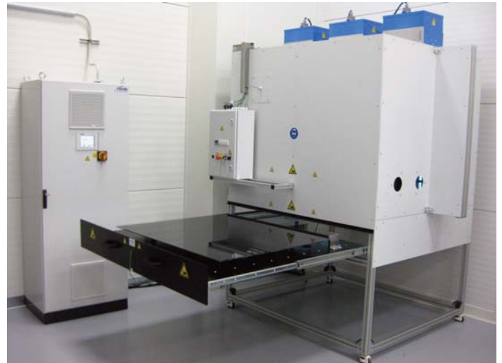
Irradiation chamber 1,1 m x 1,3 m
